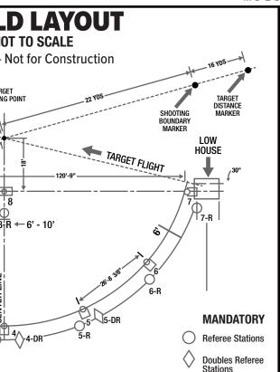
markers plus or minus six inches; target emergence elevation, high house, plus or minus three inches from level of Station 1, low house plus or minus three inchese from level of Station 7. Station levels within plus or minus nine inches of Station 8 level. Mandatory referee positions should be marked.
